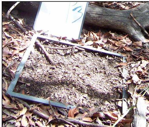
**Figure 1** Photograph of 0.5 m quadrat used to take fuel samples. (Photo: J. Gilroy)
